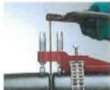
The jackbars are designed to allow clearance around the pipe for any welding torch or rod.
