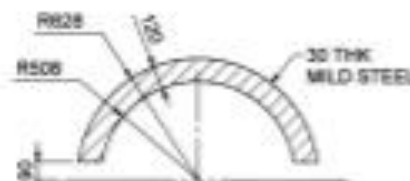
SECTION B-B REINFORCEMENT PLATE (1 OFF) SCALE 1:20
